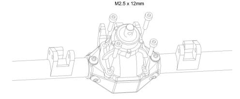
4 Use straight rear axle shafts and bearings.
