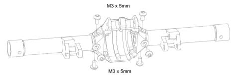
2 Install gears with the stock bearings
