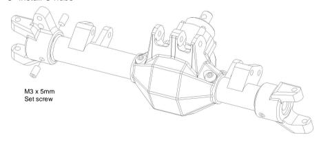
Complete the assembly using the offset universal shafts and compatible knuckles/bearings.
