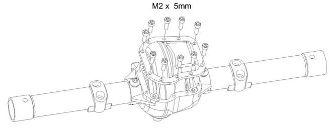
5 Install straight rear axle shafts and bearings
