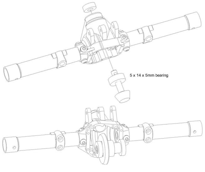
Be careful not to over tighten the screws M2.5 x 8mm
