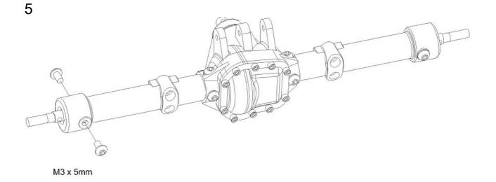
After axle assembly is complete they can be installed on the SCX10 II chassis in the same way as the stock axles.
