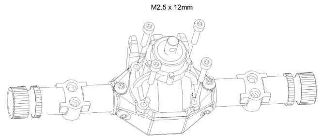
The front axle assembly (shafts, C-hubs, knuckles, link mounts) can be completed in the same way as the stock axle.
